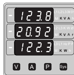
Screen 6 : System powers (Apparent, reactive, active)
