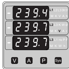
Screen 1 : Voltage Line to Neutral (For 3Ph4 Wire only)
